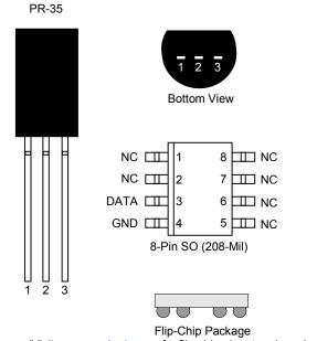
(Visit www.maxim-ic.com for flip-chip pinout and mechanical data.)
